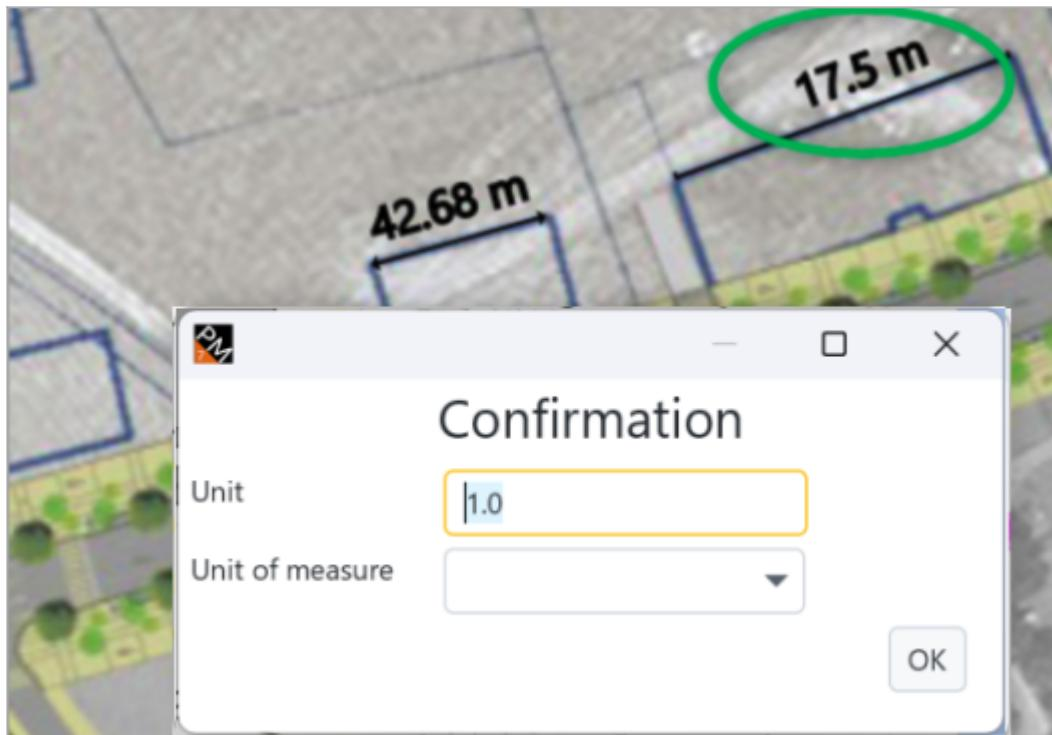
The other building's length and the track width measurements are automatically adjusted :
